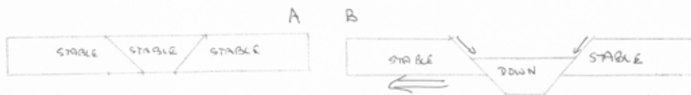
Figure: How three blocks with two “faults” cut at 45 degree angle can model extensional tectonics.
