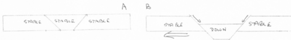
Figure: How three blocks with two “faults” cut at 45 degree angle can model extensional tectonics.
